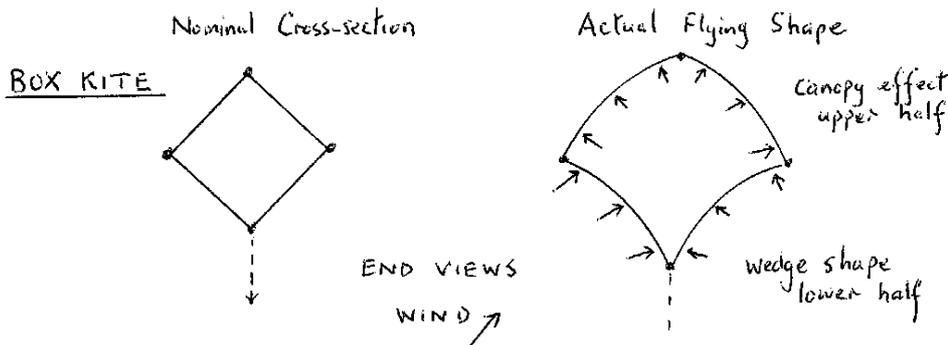
The Box Kite has a relatively inefficient wing shape (i.e. It is a combination of different shapes) but is in fact a very stable flier, because its flying surfaces are effectively 50% upward pressure and 50% sideways pressure for stability. In practice the nominally square shape is distorted under wind pressure into the effective wedge and canopy shapes.
