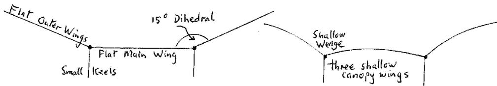
This model comprises three large square wings and although it does not have any Wedges as such, it does have generous dihedral which effectively imparts a very shallow wedge-like shape to each wing, giving the kite stability; especially a good flier in light winds.
