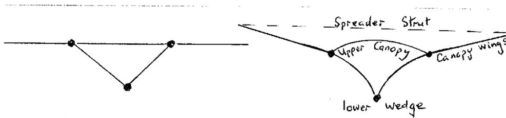
The Conyne has a distinct main wedge centre section supporting shallow or flat canopy wings. Therefore it has good flying characteristics in moderate winds. The Conyne concept is used as a main component of many other derivative designs.
