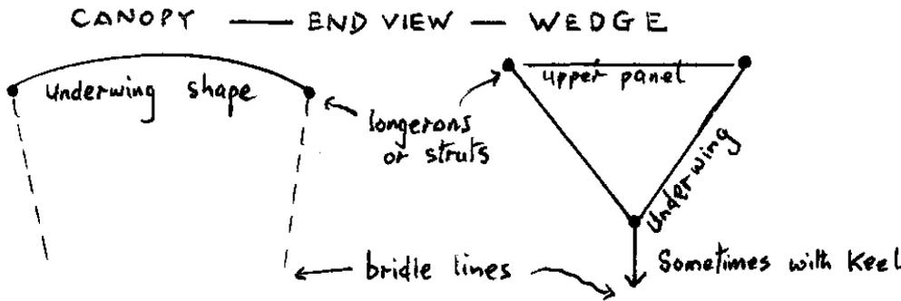
In the following explanation and drawings I refer to these shapes as being the Wedge and the Canopy. When actually flying pressure is exerted primarily in a vertical direction, but there are important side pressures on the more vertical slopes
