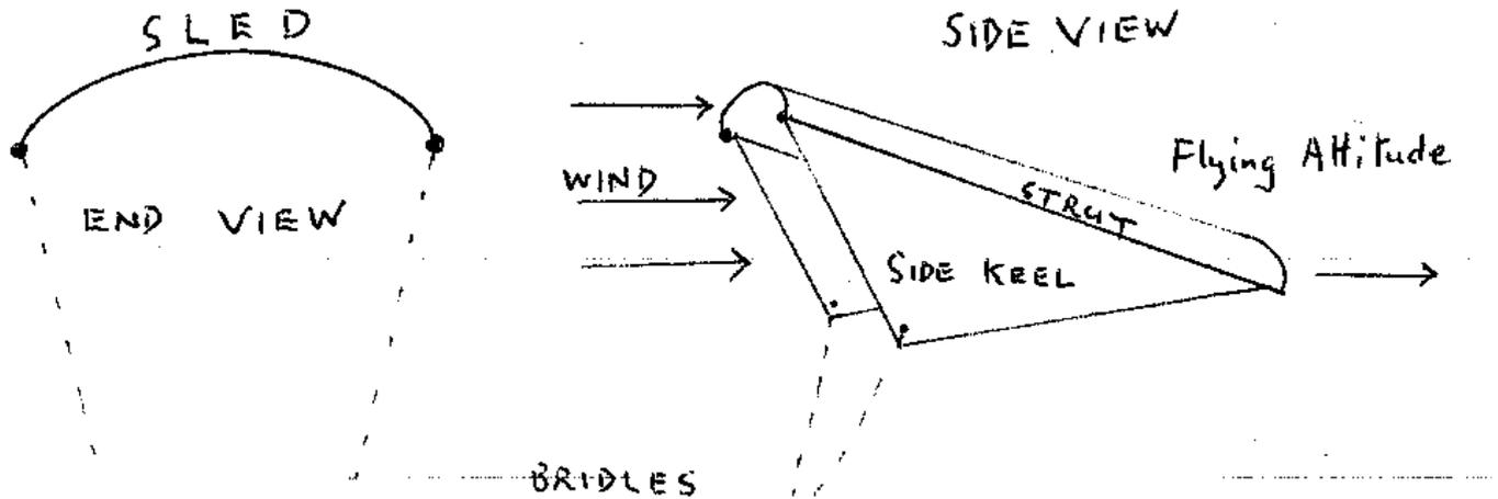
Therefore the sled design gives a comparatively flat profile front to rear (usually supported by sleeved straight spars the length of the kite), exactly contrary to the notion of an aerofoil cross section, but because of the unimpeded airflow from front to rear, the design imparts good upward pressures, which makes this simple kite a very efficient flier. There is no lift, just good airflow and upward pressure.
