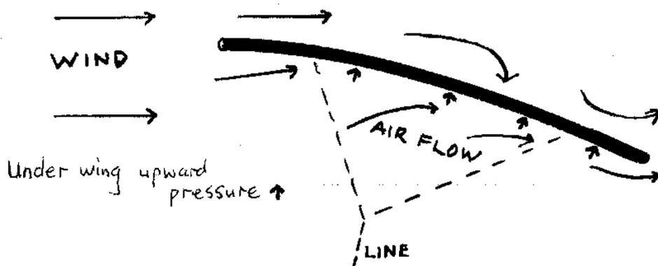
So what about the upper surface? What happens there if it is not generating *lift*? The airflow across the underside produces the essential upward pressure to billow out the shape and make the kite fly, and so react against its bridle and flying line. In choosing a shape for our kite, and in its manufacture, we primarily
