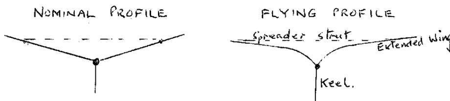
The delta is mostly a wedge shape but has canopy like outer wings. It comes in a range of plan forms of varying aspect ratios, and can therefore be adapted to various wind speeds. The spreader strut is used to determine wither a tight shallow wedge and wing or to allow a more generous deeper wedge and canopy wings.
