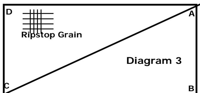
If the ripstop grain is along the length of the piece (Drawing 3) then you either have to taper from each side of the material (wastage) or cut AC and then join AD-BC – otherwise the grain will cause distortion. Furthermore you have to consider either hot cutting to seal the edges or hemming. The end of a long banner tail is notoriously prone to fraying due to the incessant vibration and movement – so at least hem the end or add a length of line *or* at least add a loop to the tip.
