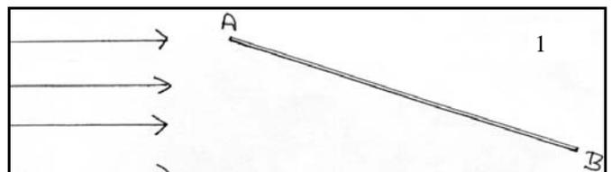
Basic Newtonian theory says that as the airflow strikes AB it will exert a force upwards which is usually called lift. If the lift is greater than the wings weight then AB will stay up. This effect is the same whether the airflow is moving at (say) 20kph against a fixed wing or the wing moves at 20kph into still air.
