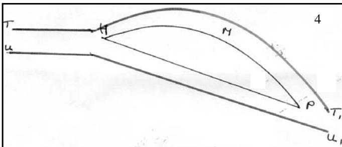
If we compare the progress of air from T to T1 and U to U1 then the top surface air must have gone faster to end up above U at U1. Now there is a very well established scientific law (Bernoulli theorem) which says that faster speed is associated with lower pressure, therefore the pressure above the wing must be lower than that below. The pressure difference is an upwards force called lift.
