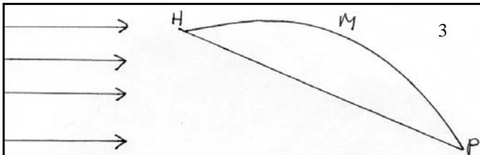
When this airfoil meets an airflow from left to right we consider what happens to two streams of air; T which follows the top hump of HMP and U which goes straight underneath from H to P.
