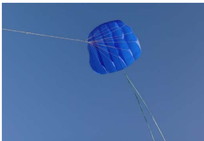
1 skin 6sq.m with bungy and pulley bridle mechanism
