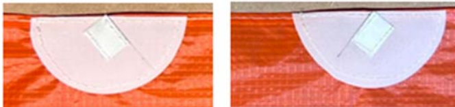
The pair of leading edge batten pockets on each side of the spine are tilted 50° towards each other, with one corner at the centre of the dacron semi circle .
