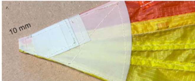
Alternative pockets for cross spar on wing tip. The lower corner of the pocket has been trimmed with the sail wing tip edges
