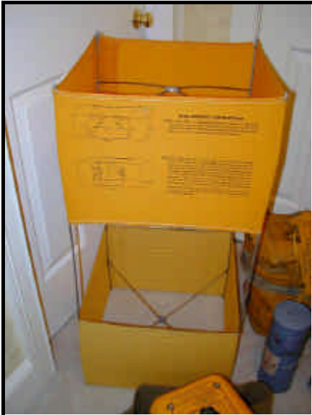
A kite from the Air-Sea rescue kit. Known to most kite fliers as the Gibson Girl it was, in fact the transmitter that the name belonged to. This is probably an American version.
