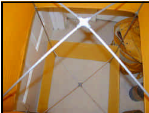
Close up of the cross spars 'umbrella' fitting. The entire kit fits in a yellow bag containing: a metal-frame box kite that folds up like an umbrella; a radio, with wire antenna to be attached to the kite; two spools of spare wire; a balloon, for use without wind; a can containing some sort of hydrogen generator for filling it; the two metal tubes may be used in the inflation process; some sort of wrench; a strobe light .
