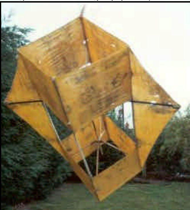
German version of the rescue kite recovered from a crashed JU88 and still flight worthy—the spars have been replaced.
