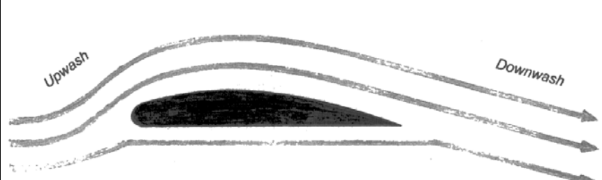
Common depiction of airflow over a wing. This wing develops no lift.
