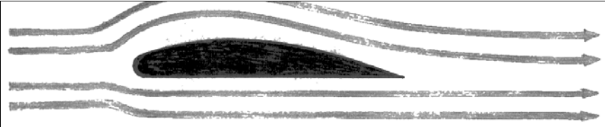
Common depiction of airflow over a wing. This wing develops no lift.
