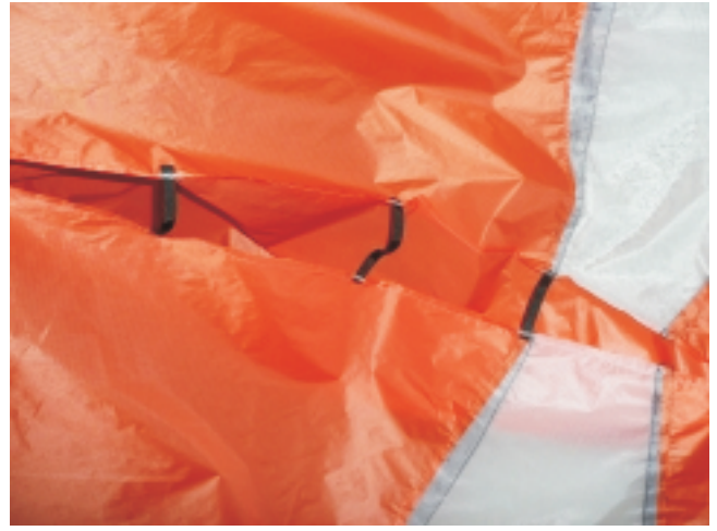
Inflation limitation of the dorsal fin by lengths of belt webbing. Reinforcement strings also work.
