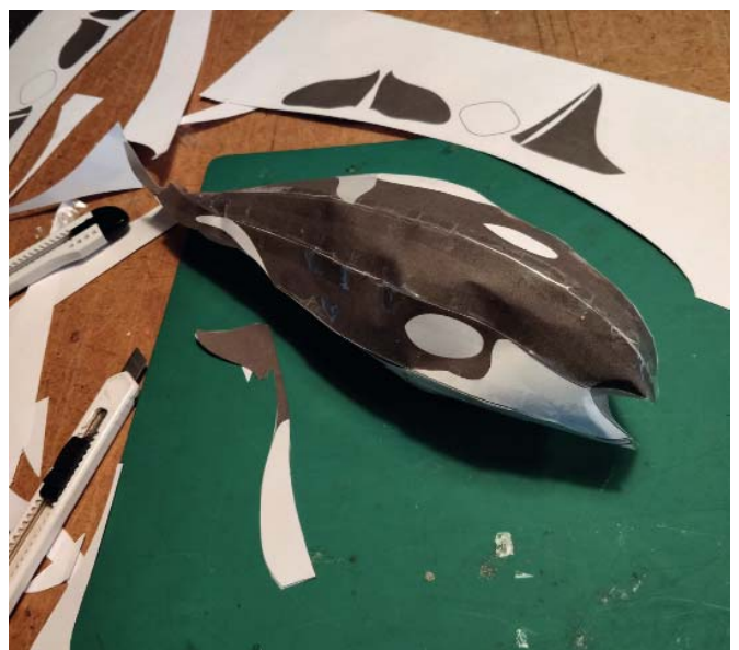
Paper testing. After designing I printed some parts out on paper to see if the idea would work. Glued some parts and it seemed to work. So work started at the first prototype.
